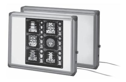
Silver-grey quality aluminium housing with grey salient angles  $\bullet$  Front panel made of acrylic glass  $\bullet$  All-around film holding rail for maximum viewing comfort  $\bullet$  Supply voltage 230 V / 50 Hz  $\bullet$  Lowering of the luminance down to 500 cd/m<sup>2</sup>  $\bullet$  Screwless front for installation and service easily removable.
